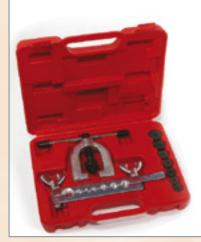
Double flares soft steel tubing up to .040 (1 mm) wall thickness. Single flares soft copper, aluminium and brass tubing. Includes hardened bar assembly with seven threaded dies  $-(1/2)^n$ , 1/4, 4.75mm. 5mm, 6mm, 8mm and 10mm) - yoke with swivel tip and sliding T-bar and seven double flare adaptors (same sizes as dies). Set is packed in heavy blowmould box and includes instructions.
